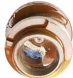
Figure 5: Accumulation in a single-vane impeller
