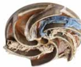
Figure 6: Accumulation in a vortex impeller
