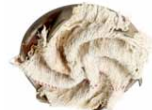
Figure 7: Accumulation in a vortex impeller
