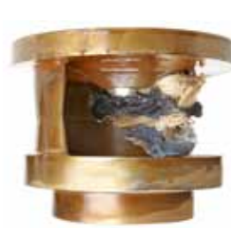
Figure 4: Accumulation in a single-vane impeller
