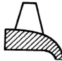
Fig. 6 Single or multistage pumps with mixed flow and propeller-type impellers have very high capacities and deliver very low heads. Specific speed range is 6000 to 10,000.
