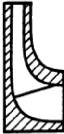
Fig. 2. Single suction, horizontal or vertical centrifugal pumps with narrow port impellers have low capacities and deliver high heads. Specific speed range is 500 to 1000.
