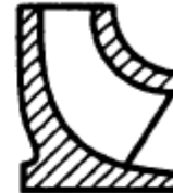
Fig. 4 Single or multistage, and single (illustrated) and double suction, Francis-type impellers, operating in volute or diffuser type casings produce medium to high capacity at medium to low speeds. Specific speed range is 2000 to 4000.
