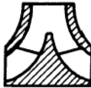
Fig. 3. Single or multistage, double (illustrated) and single suction, volute and diffuser design centrifugal pumps deliver medium capacity and medium heads. Specific speed range is 1000 to 2000.
